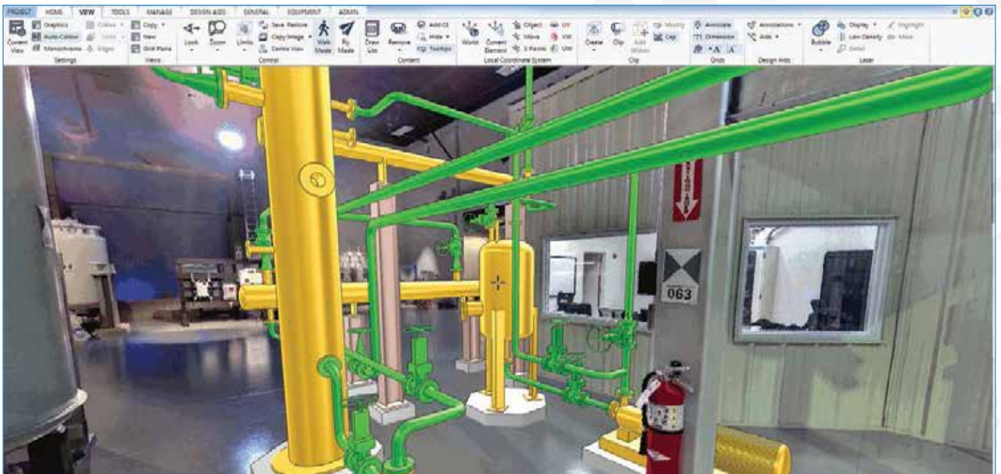
Photorealistic BubbleView™ laser scan viewing technology in AVEVA E3D enables piping design to be carried out in the context of the as-built facility
